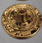
6.) Install OD piston and return spring. Torque the pump assembly bolts.(23 ft.lb.)
