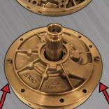
fig. b and flip over onto remaining pump half. Aligning oval hole to pump filter.
