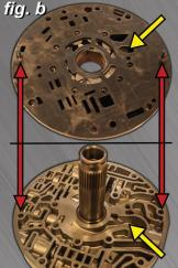
2.) Lay plate over pump body, oval hole to oval pathway end.
