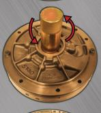
5.) Use pump alignment tool to center both halfs, turn it slowly until you feel it drop, with one hand on the pump alignment tool and the other under the pump, flip the unit over.
