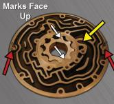
1.) Lay pump body face up, install alignment pins from bottom side in the proper holes.
